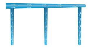
Since the air velocity in main duct of UR system is completely stable and balanced while the included angle between duct surface and branch duct is slightly less than 90°, that is conducive to lead uniform air distribution to each branch.
