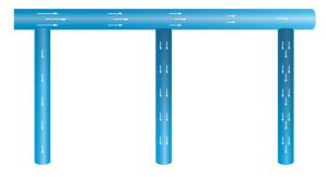
Different air velocity in main duct of Ordinary equant round fabric duct leads to different airflow supply in each branch, which causes the nearer the branch is to endcap, the more airflow the branch is to receive. ACD is required to balance airflow in each branch.
