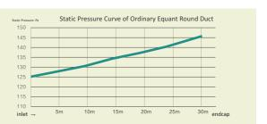
Since UR system is cone-shaped from inlet to endcap, its on-way resistance is larger than that of ordinary equant round duct. Meanwhile, the internal air velocity is relatively uniform and the static pressure regain is lower. The test result turns out that UR system could basically achieve balanced inner static pressure as long as it is not exceptionally long.
